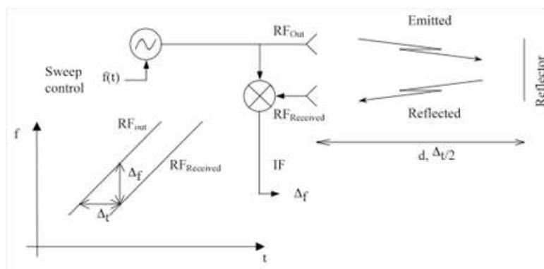
Figure 1. Schematic presentation showing how a low frequency signal is generated by mixing the received RF signal with the output RF signal. Due to the delay,  $\Delta t$ , caused by emitted signal
