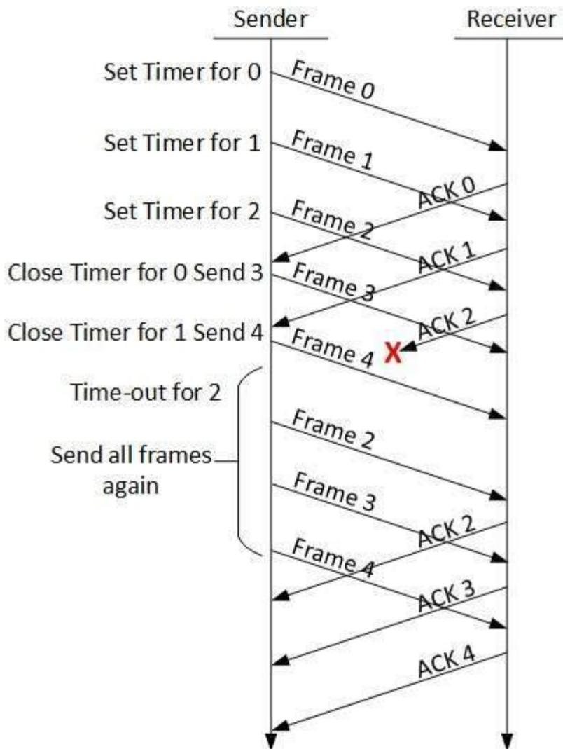
The sending-window size enables the sender to send multiple frames without receiving the acknowledgement of the previous ones. The receiving-window enables the receiver to receive multiple frames and acknowledge them. The receiver keeps track of incoming frame's sequence number.
