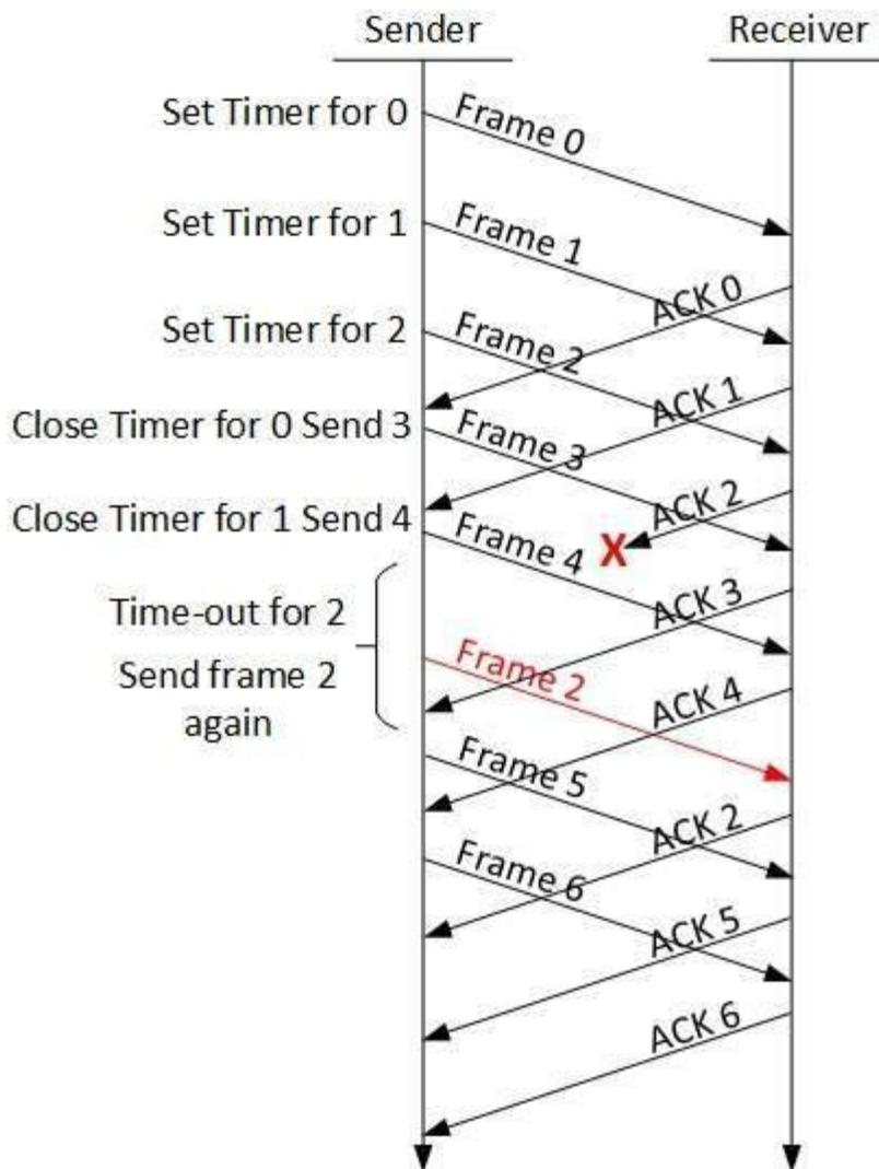
In Selective-Repeat ARQ, the receiver while keeping track of sequence numbers, buffers the frames in memory and sends NACK for only frame which is missing or damaged.
