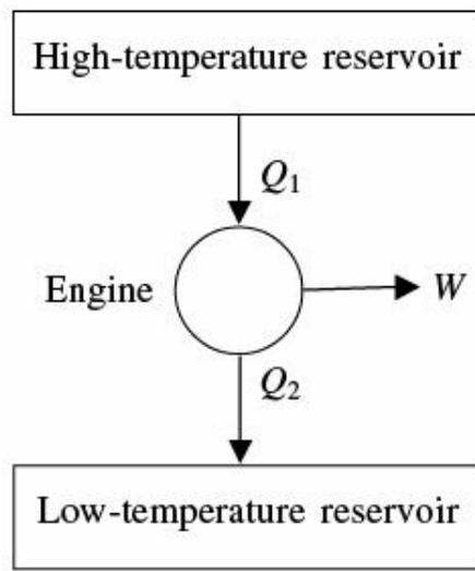
**Fig. 1.3** Schematic representation of a heat engine.
