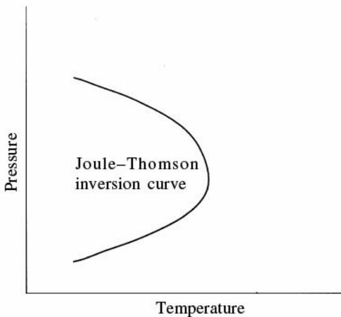
**Fig. 6.6** A typical Joule–Thomson inversion curve.
