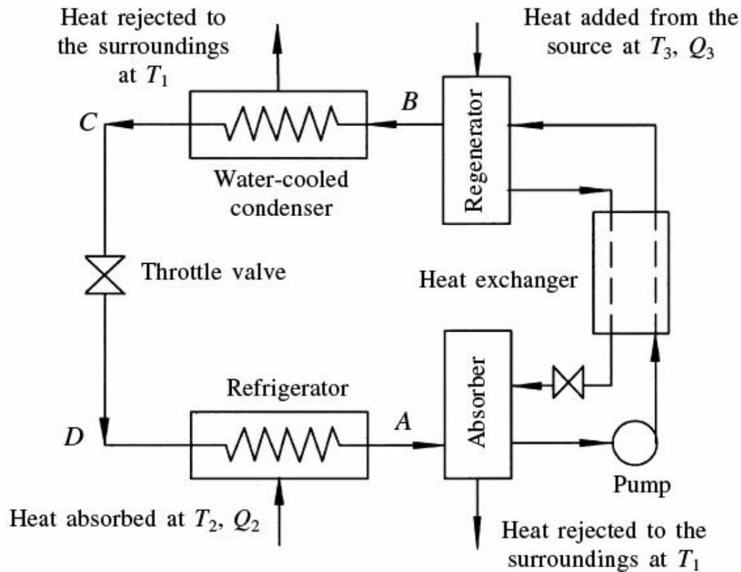
**Fig. 5.14** Absorption refrigeration cycle.
