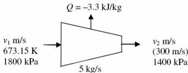
**Fig. 2.6** Flow through nozzle in Example 2.15.
