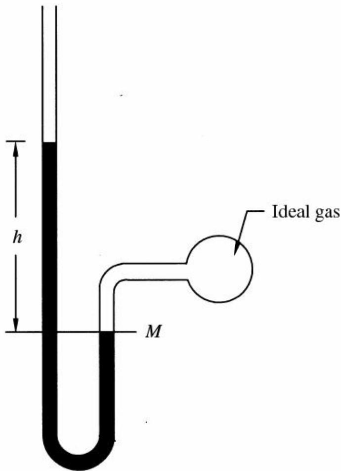
**Fig. 1.2** Constant-volume gas thermometer.
