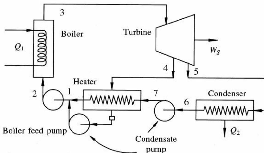
**Fig. 5.22** Components of a regenerative cycle.
