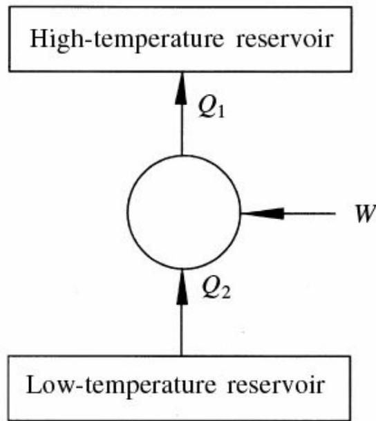
**Fig. 5.7** Schematic representation of a refrigeration cycle.
