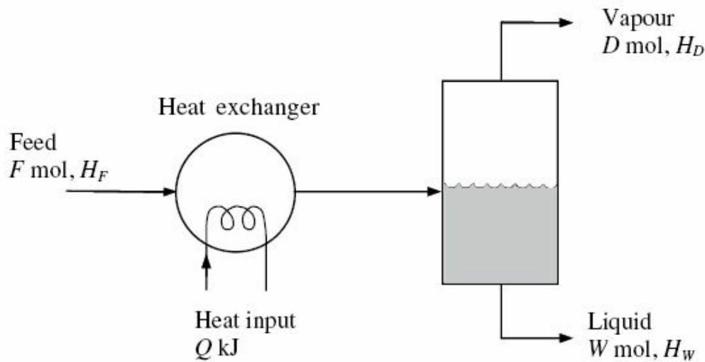
**Fig. 2.5** Flash vaporisation process in Example 2.12.
