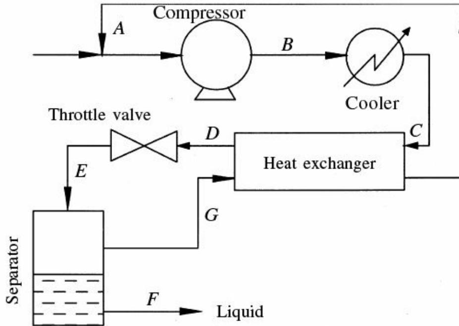
**Fig. 5.16** The Linde process for gas-liquefaction.
