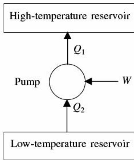
**Fig. 1.4** Schematic representation of a heat pump.
