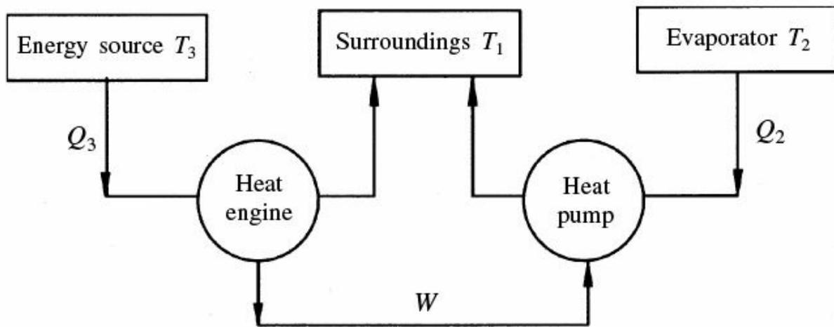
**Fig. 5.13** The principle of absorption refrigeration.
