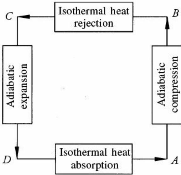
**Fig. 5.8(a)** Components of a Carnot cycle.
