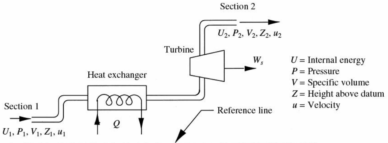
Fig. 2.4 Steady-state flow process.
