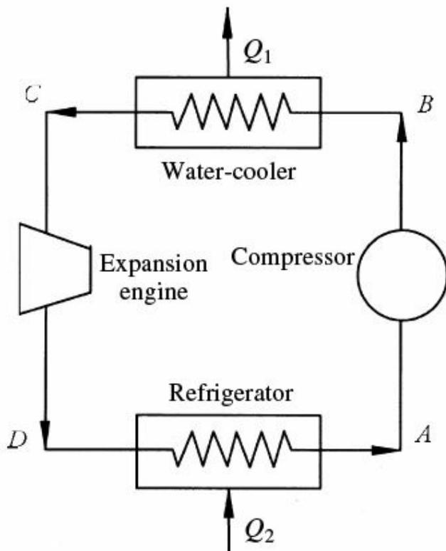
**Fig. 5.12(a)** Components of an air-refrigeration cycle.
