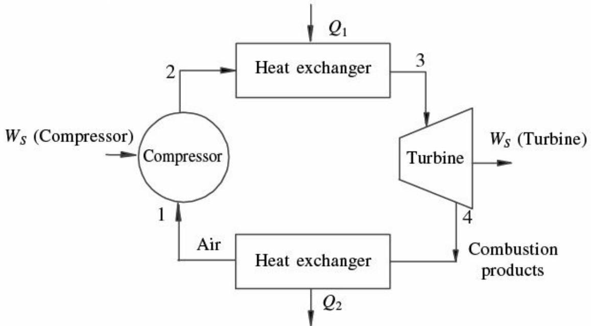
**Fig. 5.27(b)** The closed cycle gas-turbine power plant.
