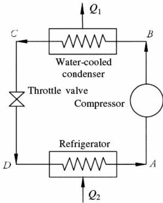
**Fig. 5.9(a)** Components of an ordinary vapour-compression cycle.
