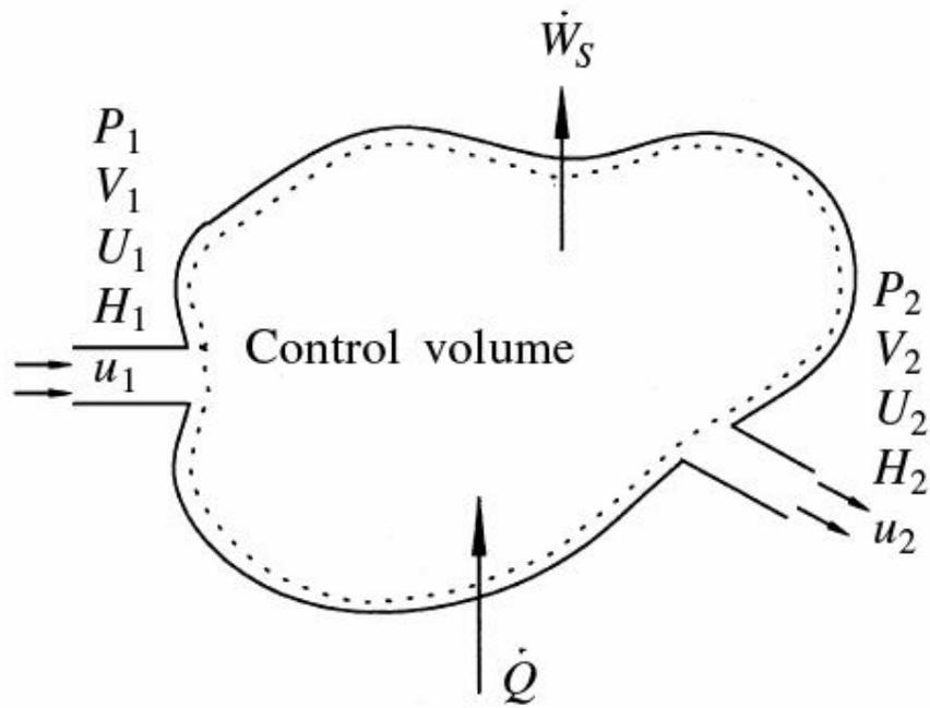
**Fig. 5.1** Energy balance for a control volume.
