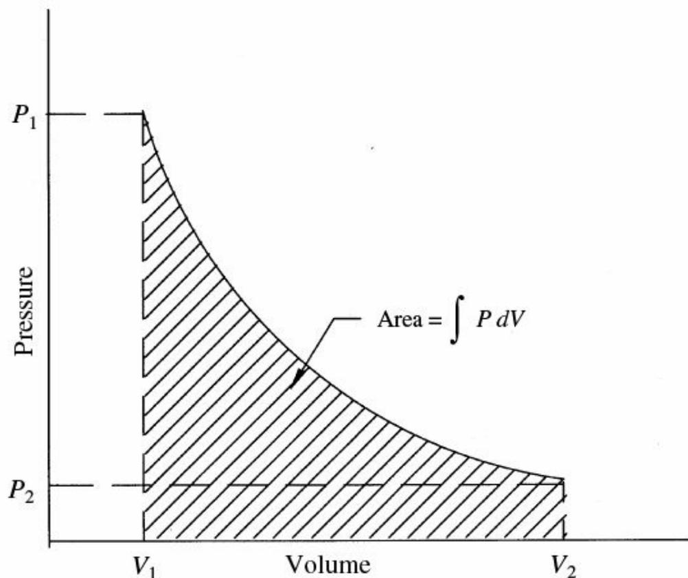
**Fig. 1.1** Work of expansion on the  $P$ - $V$  diagram.
