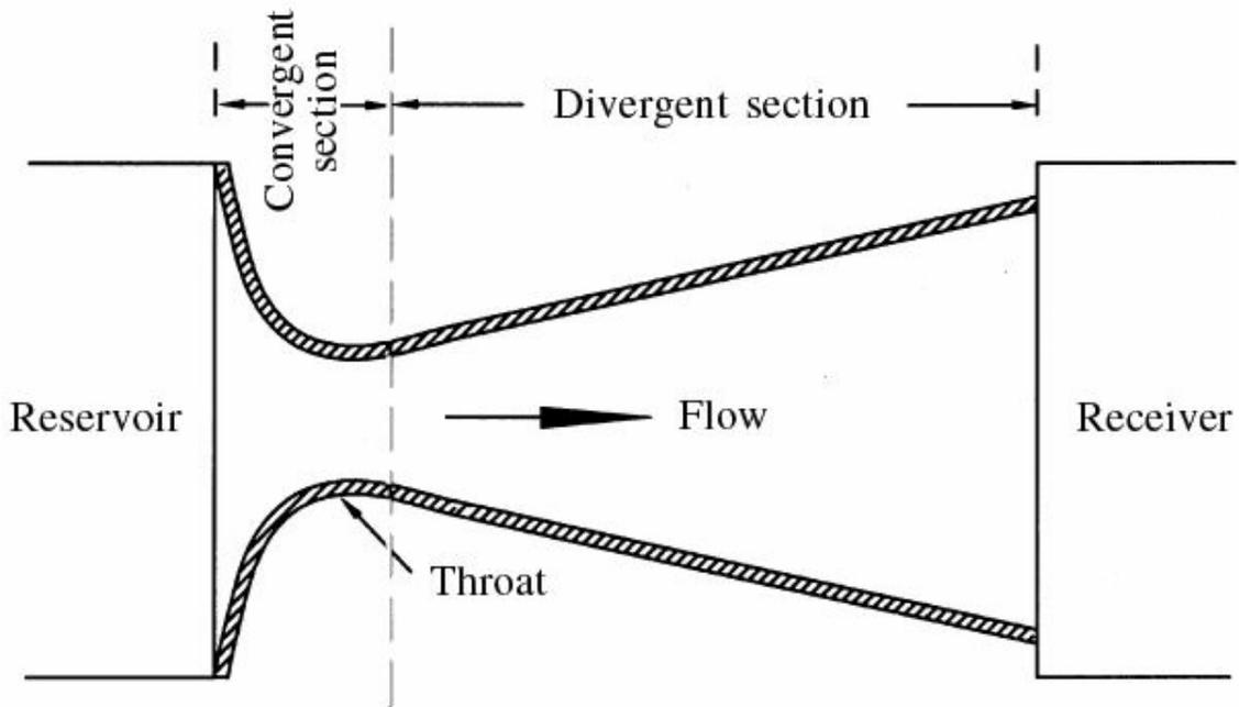
**Fig. 5.2** The convergent-divergent nozzle.
