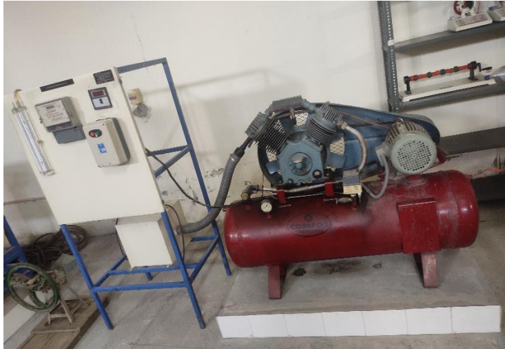
Two Stage Air Compressor Test Rig
